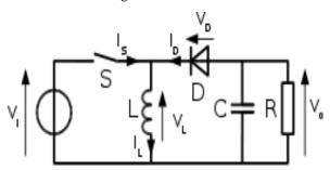
While in the On-quality, the input voltage source is directly connected to the coil (L). This arise in accumulating energy in L. In this stage, the capacitor supplies energy to the product lading. While in the Offstate, the coil is connected to the output load and condenser, so spirit is pass from L to C and R.
